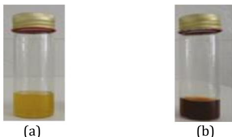
Figure 1. Color changes of Stachys lavandulifolia vahl extract (a) before reaction and after reaction with silver nitrate ( \text{AgNO}_3 )
